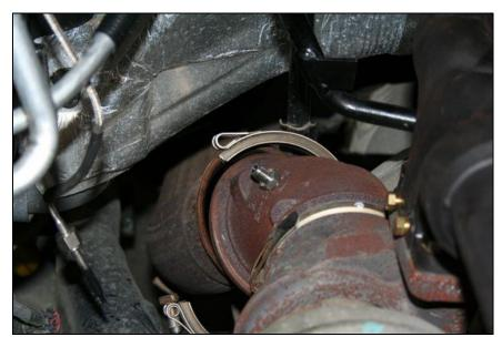
Disconnect the compressor outlet boot.
