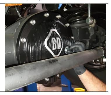
Some differentials may require special additives, please check your owner's manual before filling. Drive at least 50Kms (31 miles) re-torque bolts to specification ensure there are no leaks. Installation is complete.
