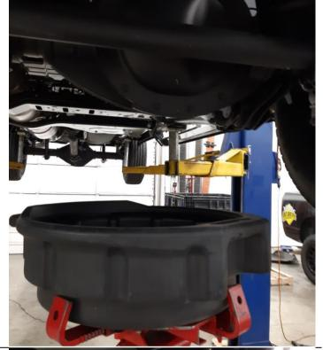
Remove bolts starting at the bottom. Leave the top bolts installed loosely, pry cover away from the housing and allow fluid to drain.
