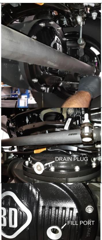
Insert fill plug (1401557) do not overtighten (9mm Allen wrench)
