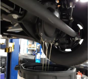
Once drained, remove cover and check differential housing gasket surface for irregularities and remove high spots if required. Surface must be flat and clean.
