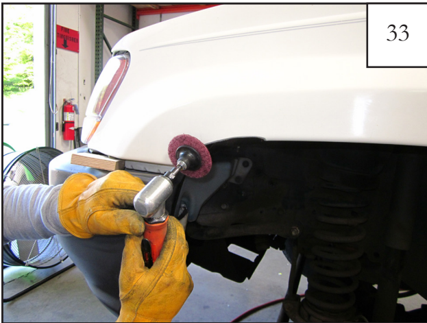
Using an angle grinder or sandpaper, sand the chipped paint along cut edge of the wheel well.
