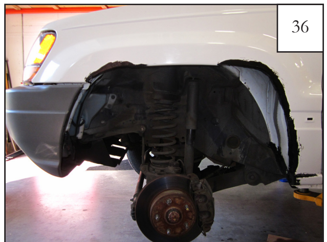
Completed cut-out with caulking applied.
