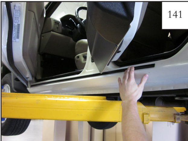
Remove tape liner from molding (GP1-0020) and starting at front hole, install molding along rocker area to cover holes in sheet metal.
