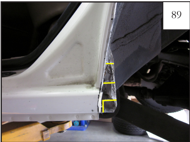
Mark vehicle for cutting: Make horizontal marks on the inner pinch weld flange approximately 1-1/2" apart.
