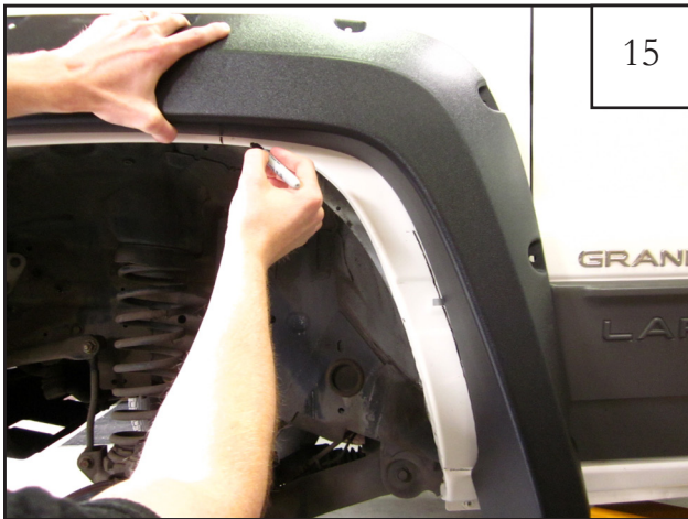
15 Hold the flare up to the fender as a guide. Make a line connecting the marks made in steps 13 & 14.
