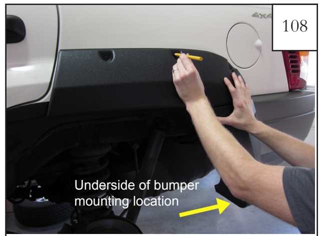
Hold flare in place on vehicle. Using an awl or grease pencil, mark hole locations onto fender through holes drilled in pockets of flares. Also mark mounting hole location on underside of bumper piece.
