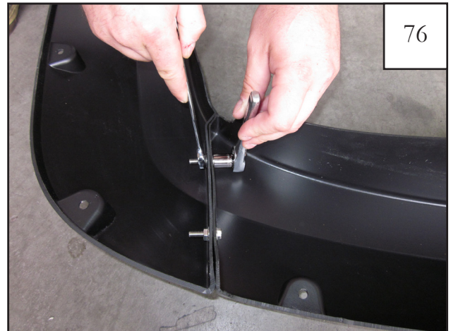
Once satisfied with alignment, tighten all screws.
