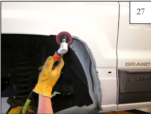
Using an angle grinder or sandpaper, sand the chipped paint along bent edge of the wheel well.
