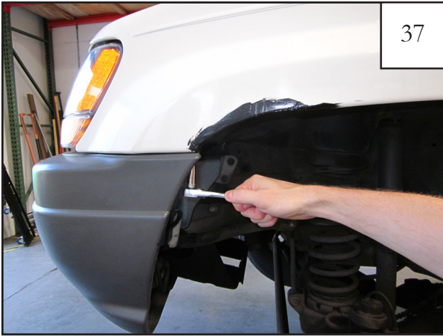
Using a 10mm socket & wrench, re-install factory screw attaching bumper to fender.
