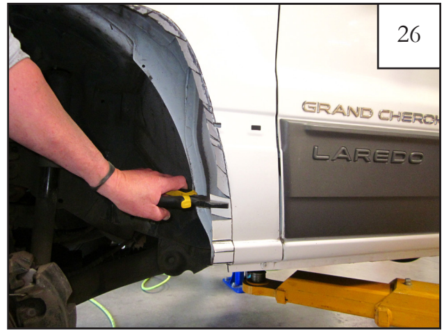
Use pliers to bend back horizontal sheet metal tabs. Use a hammer to flatten out sheet metal tabs. Avoid bending or distorting outer sheet metal.
