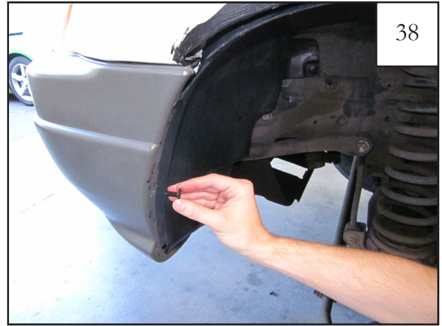
Re-install splash shield using supplied panel retainers (RV1-P008). See next step for retainer locations.
