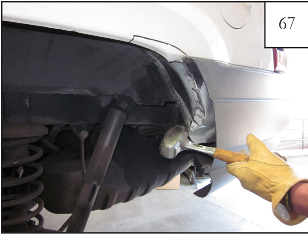
Using a hammer, pound the tabs made in the inner sheet metal flat against wheel well.
