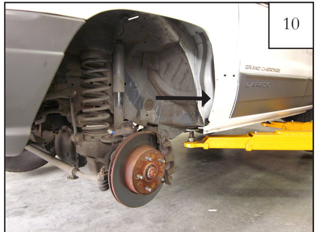
10 Remove splash shield and push sound dampening foam back into inner wheel well behind the fender. NOTE: If debris is present in inner wheel well, remove before continuing installation.
