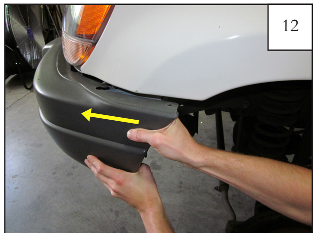
12 Push front bumper forward away from wheel well to release from factory installed clip in fender.
