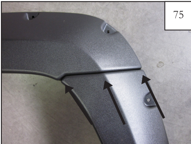
Check alignment of main flare and bumper piece to each other. Line up the three style lines.
