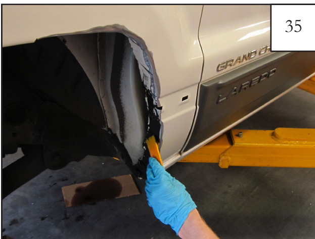
Apply urethane caulking or primer to seal any exposed sheet metal for rust prevention.
