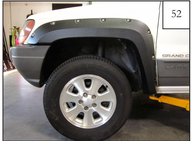
Completed front flare installation.
