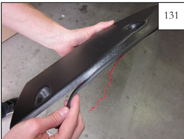
For edge trim application on rear door piece, follow steps as listed at the beginning of this instruction. Apply edge trim (GP1-0005) only to the outer edge of the door piece.
