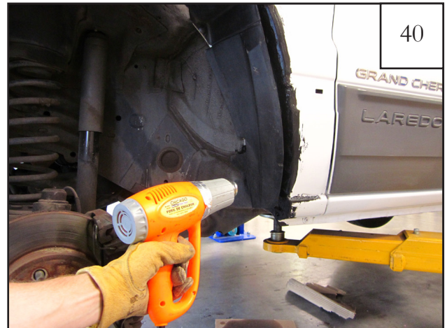
Using a heat gun, heat splash shield until pliable and use heavy work gloves to push and mold splash shield into place aligning with trimmed inner wheel well. Hold it in place and allow to cool. Then fully install push retainers in splash shield.
