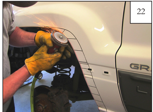
Using a cut off wheel or other suitable tool, cut along line marked in step 21 removing the inner flange.
