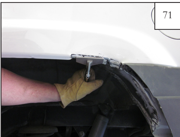
Use sheet metal pliers to bend straightened tabs back and up into wheel well.
