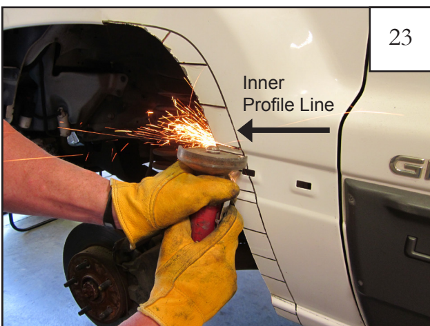
Using a cut off wheel or other suitable tool, cut along horizontal marks from wheel well to inner cut profile line.
