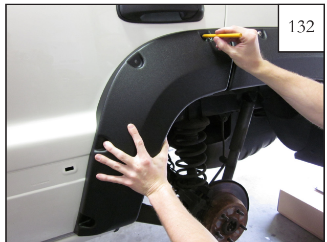
Press door piece firmly against vehicle aligning with rear main flare. Mark hole locations on fender through holes drilled in pockets of door piece. Parts are marked on the inside. Driver's side: D1 for door piece.
