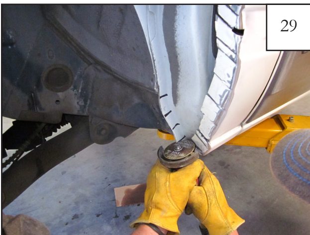
Using a cutoff wheel or other suitable tool, starting at the bottom line, cut horizontal marks in the pinch weld.
