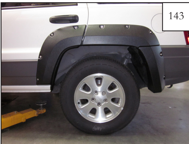
Completed rear flare installation.
