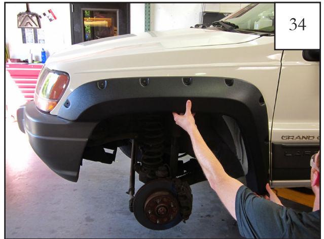
Hold flare up to wheel well to confirm fit. Make adjustments to cut as needed.
