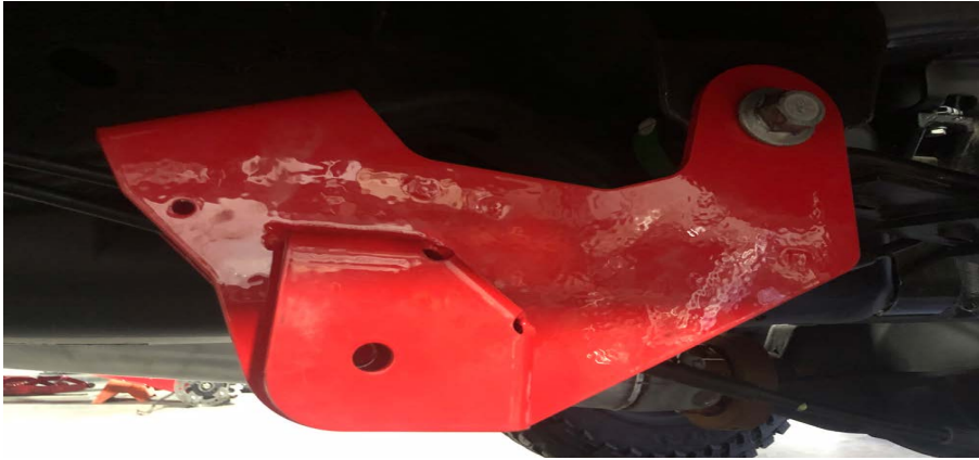
Figure 3: Mount Frame Mount Bracket
