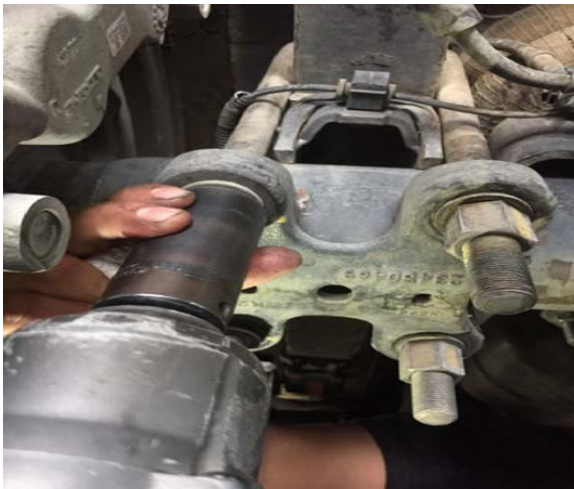
Figure 25: Remove U-Bolt Nuts
