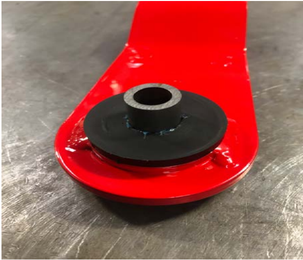
Figure 17: Install Shackle Crush Sleeves
