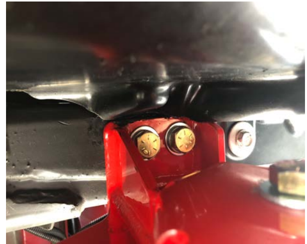
Figure 13: Fuel Tank Shield Trimmed
