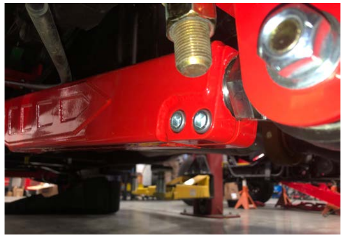
Figure 37: Adjuster Nut Clamp
