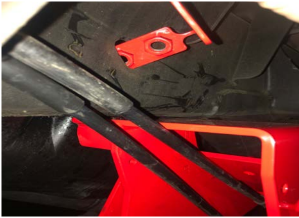
Figure 10: Insert Nut Plate
