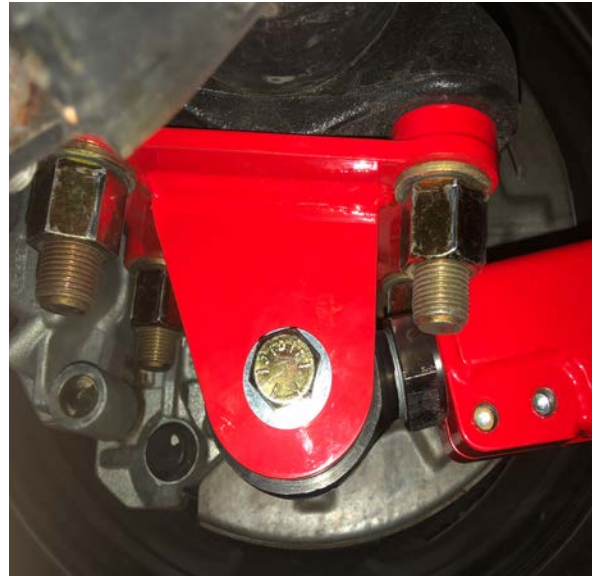
Figure 35: Traction Bar Rod End / Rear Axle Pivot
