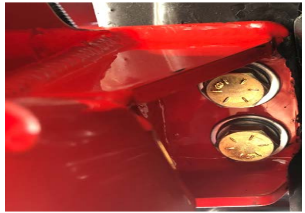
Figure 11: Install Front Frame Mount Hardware
