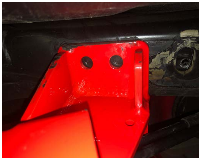
Figure 5: Frame Mount Bracket Location
