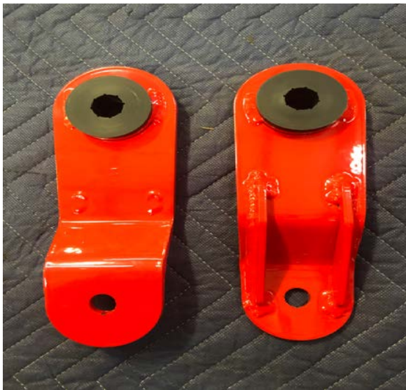
Figure 15: Install Shackle Bushings
