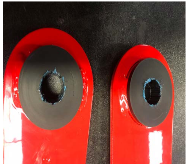
Figure 16: Grease Shackle Bushings
