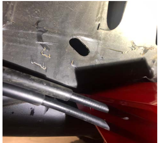
Figure 9: Nut Plate Window
