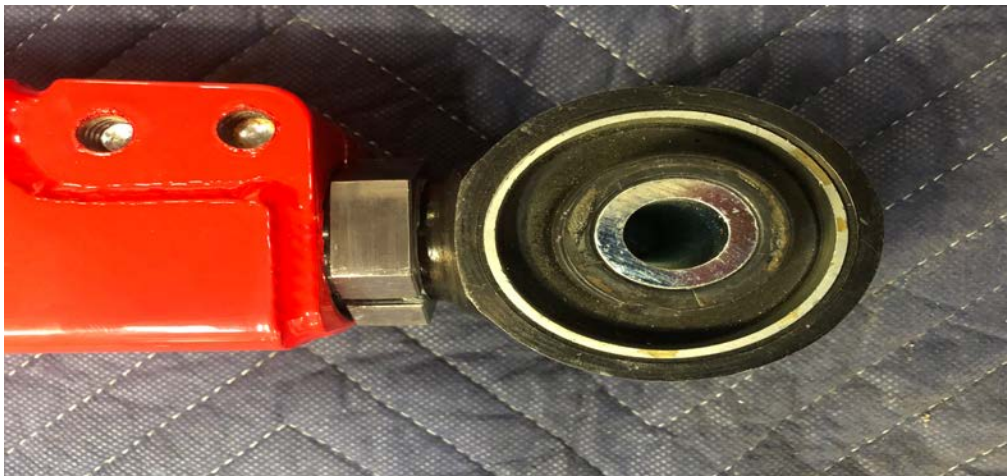
Figure 33: Traction Bar Rod End
