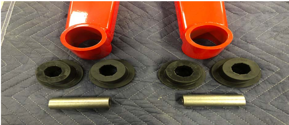
Figure 27: Traction Bar Bushing Parts
