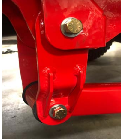
Figure 32: Traction Bar / Shackle Pivot
