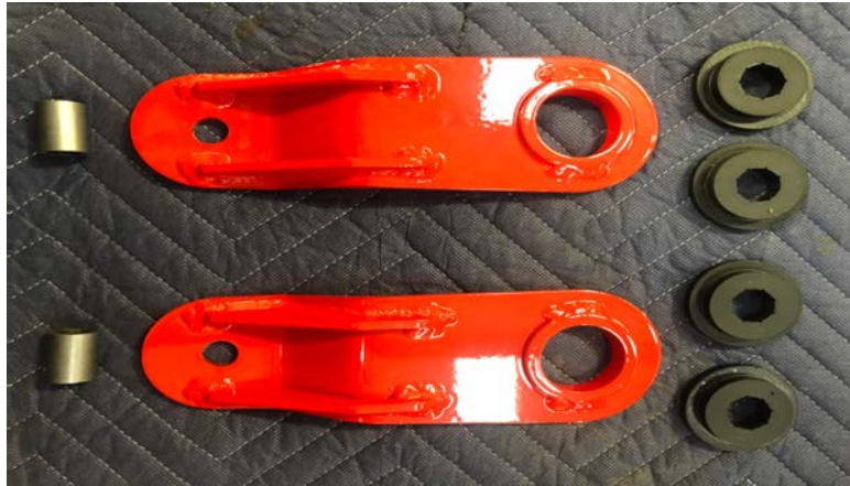
Figure 14: Traction Bar Shackle Parts
