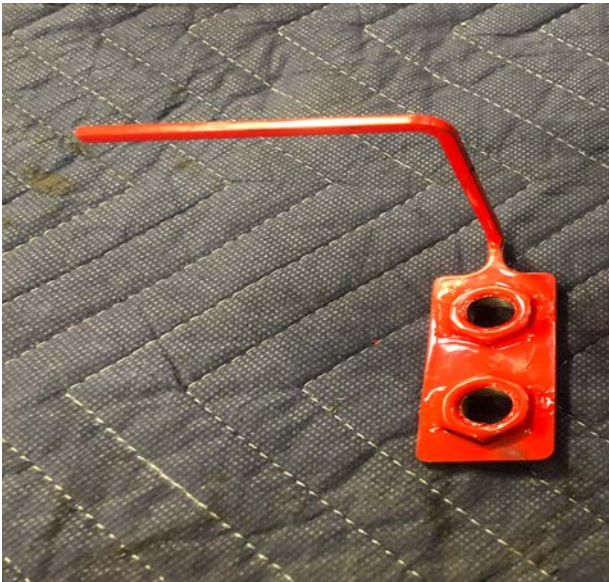
Figure 8: Nut Plate (Driver Side)
