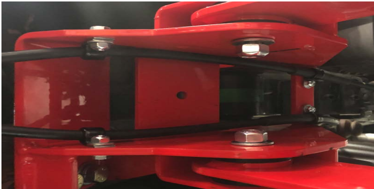
Figure 21: Route Brake Cables
