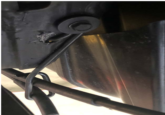
Figure 1: Remove Brake Cable Bracket
