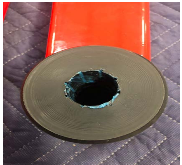
Figure 29: Traction Bar Bushings Greased
