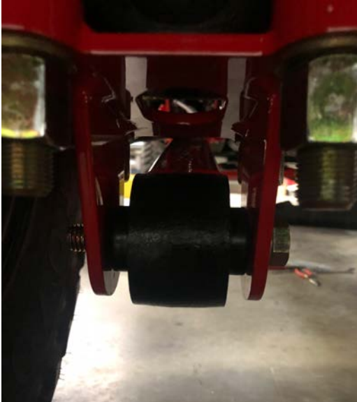
Figure 34: Traction Bar Rod End / Rear Axle Pivot
