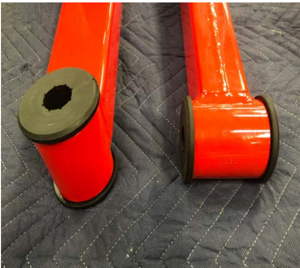
Figure 28: Traction Bar Bushings Installed
