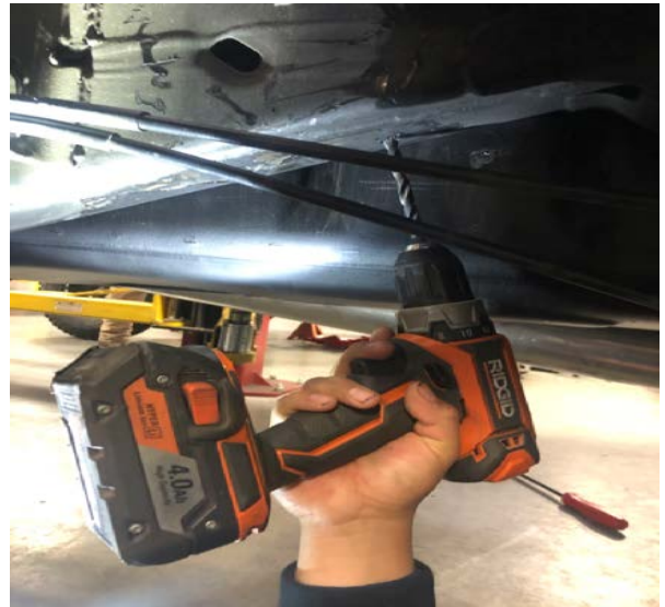
Figure 7: Drill Frame Mount Holes
