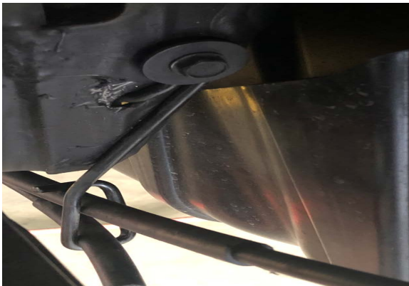
Figure 1: Remove Brake Cable Bracket
