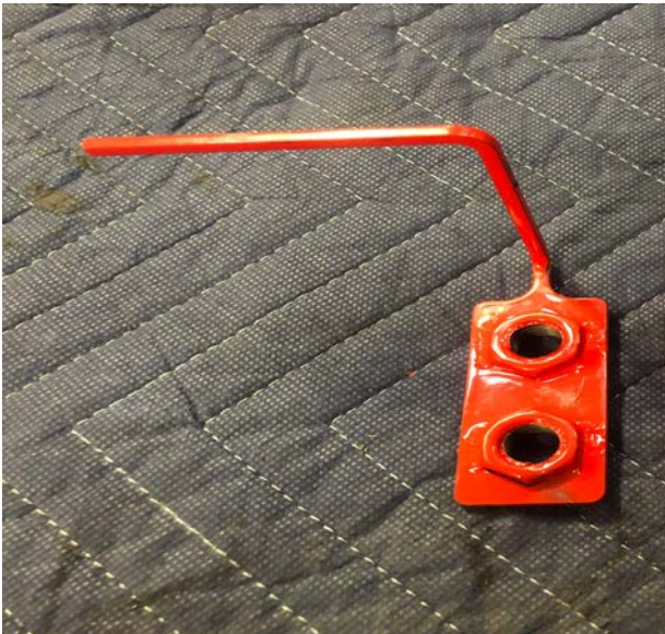
Figure 8: Nut Plate (Driver Side)
