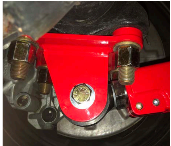
Figure 35: Traction Bar Rod End / Rear Axle Pivot
