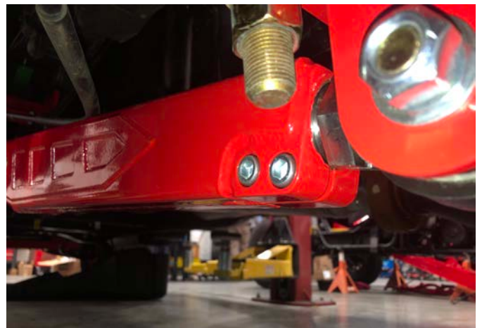
Figure 37: Adjuster Nut Clamp
