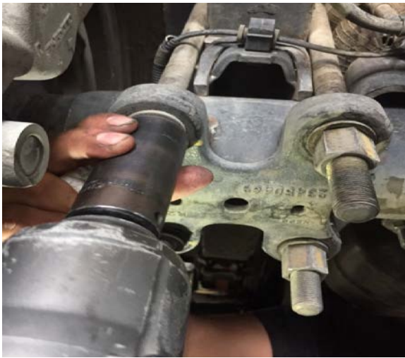
Figure 25: Remove U-Bolt Nuts
