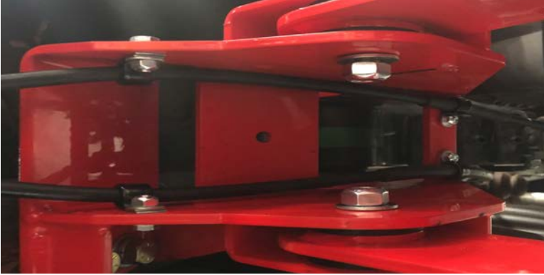
Figure 21: Route Brake Cables
