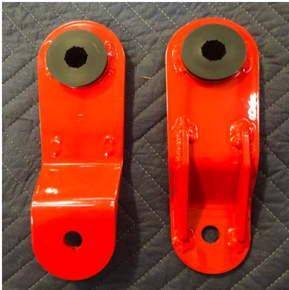
Figure 15: Install Shackle Bushings
