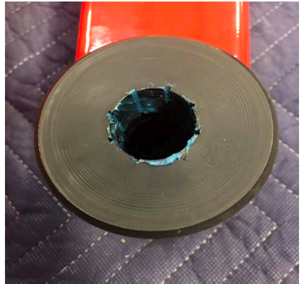
Figure 29: Traction Bar Bushings Greased
