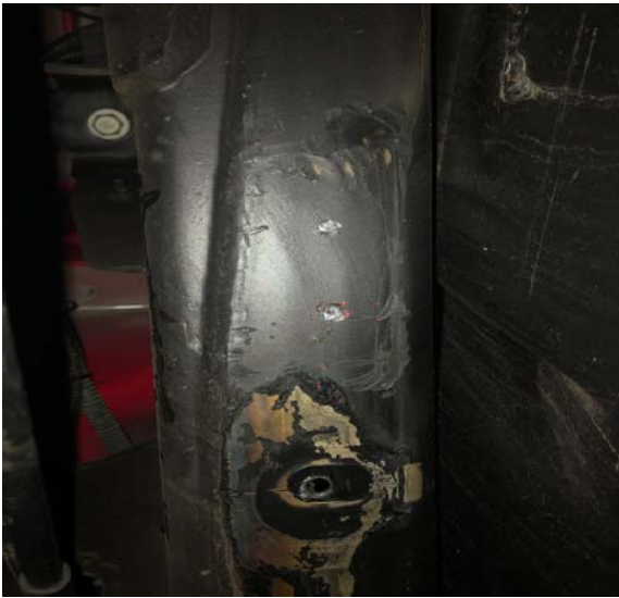
Figure 6: Frame Mount Hole Locations
