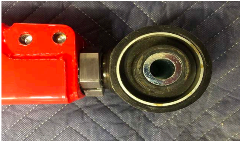
Figure 33: Traction Bar Rod End
