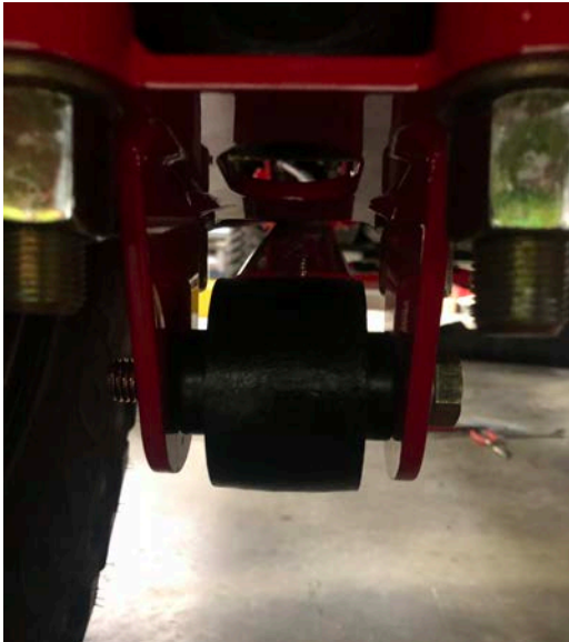
Figure 34: Traction Bar Rod End / Rear Axle Pivot
