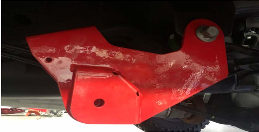
Figure 3: Mount Frame Mount Bracket
