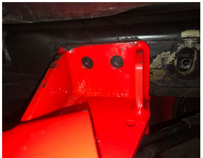
Figure 5: Frame Mount Bracket Location
