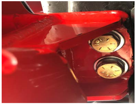
Figure 11: Install Front Frame Mount Hardware
