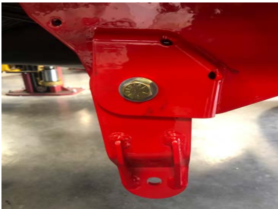
Figure 19: Assemble Shackles to Frame Mount
