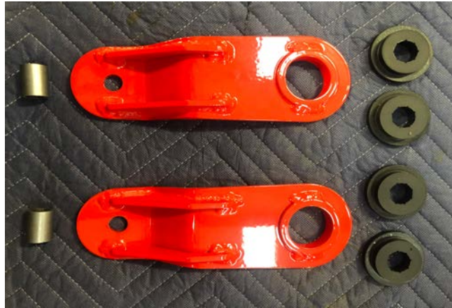
Figure 14: Traction Bar Shackle Parts
