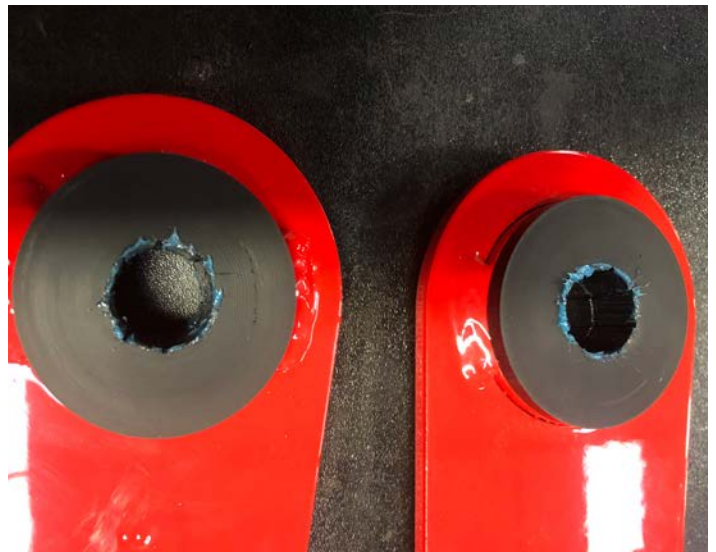
Figure 16: Grease Shackle Bushings
