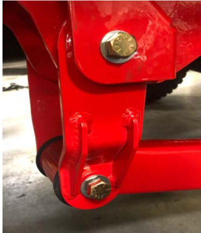
Figure 32: Traction Bar / Shackle Pivot
