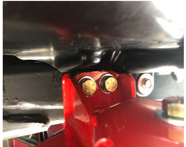
Figure 13: Fuel Tank Shield Trimmed
