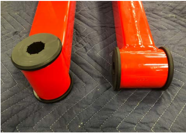
Figure 28: Traction Bar Bushings Installed
