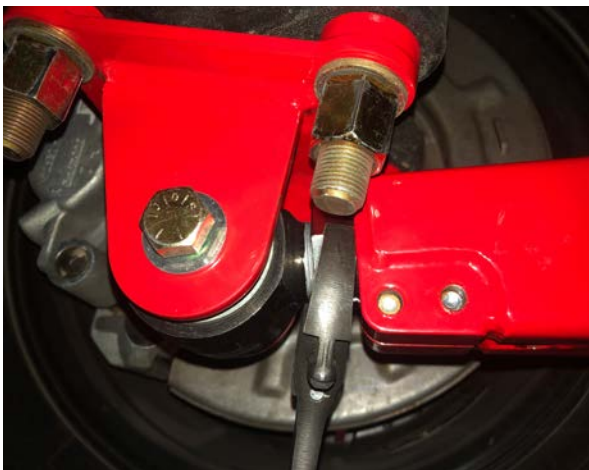
Figure 36: Traction Bar Length Adjustment
