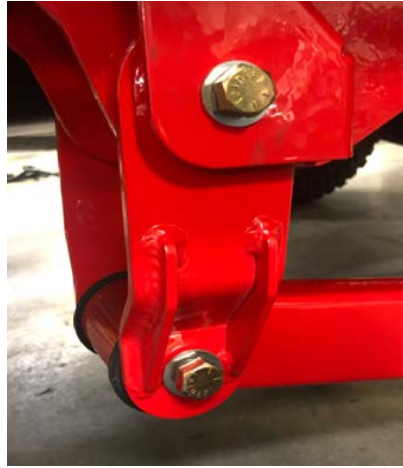
Figure 32: Traction Bar / Shackle Pivot
