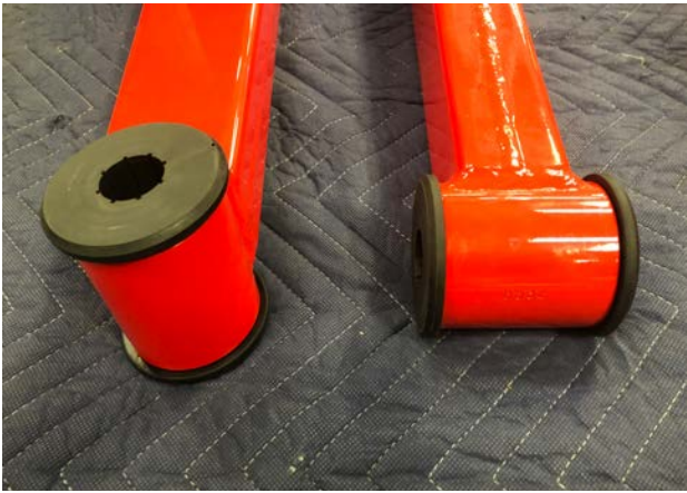
Figure 28: Traction Bar Bushings Installed
