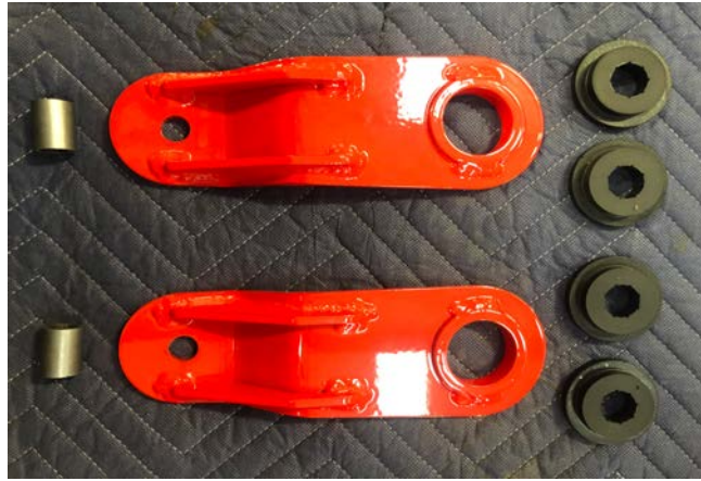
Figure 14: Traction Bar Shackle Parts
