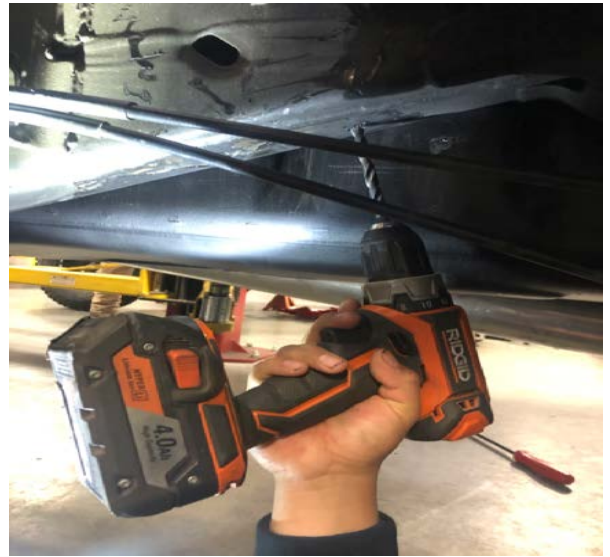
Figure 7: Drill Frame Mount Holes
