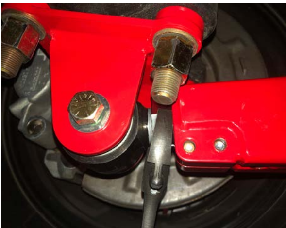
Figure 36: Traction Bar Length Adjustment
