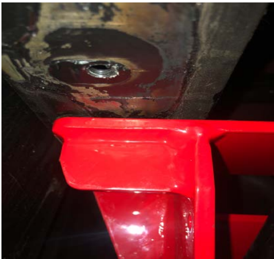
Figure 4: Frame Mount Bracket Location
