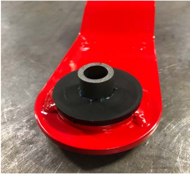
Figure 17: Install Shackle Crush Sleeves
