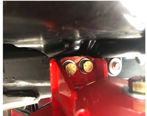
Figure 13: Fuel Tank Shield Trimmed
