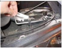
Step 2: Pull the pin straight out to loosen the headlight assembly.
