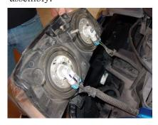
Step 4: Disconnect the headlight wire harness from the high and low beam light bulbs.
