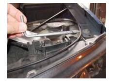
Step 3: Pull the headlight straight out of the housing.
