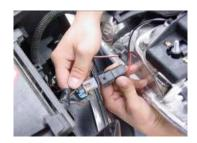
Step 7: Connect the headlight plugs into the new headlight.
