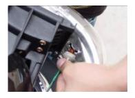
Step 9: Plug and twist the turn signal light into the new headlight
