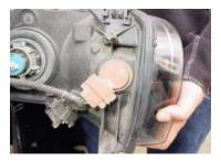
Step 6: Pull the turn signal socket out of the housing.
