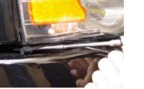
Step 3: Remove the bolt located underneath the headlight.
