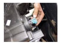
Step 9: Plug the headlight socket to the bulb.
