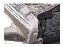
Step 1: Remove the plastic screws to remove rubber shroud.
