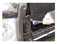
Step 2: Remove the upper and lower 10mm bolts.
