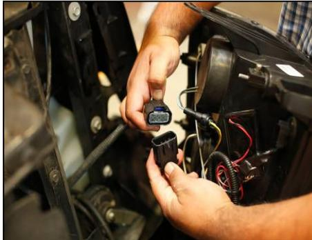
Disconnect main wiring harness from factory headlight.
