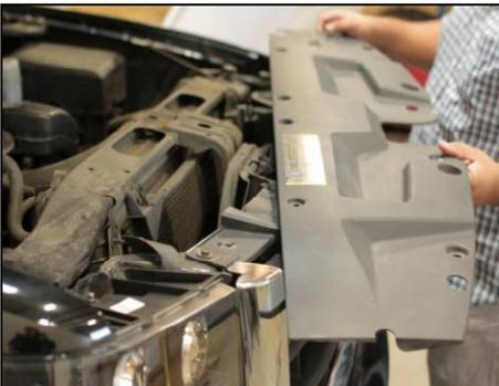
Remove factory radiator shroud and set aside.
