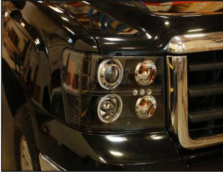
**Slide headlight into bucket and reverse steps 10-12 to install headlight.**
