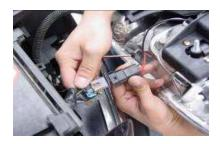
Step 7: Connect the headlight plugs into the new headlight.
