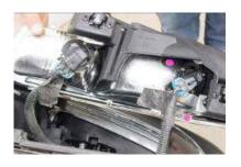
Step 3: remove the headlight connecters for the high and low beam.
