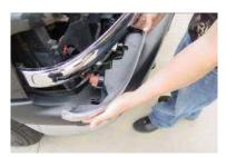
Step 4: take off the turn signals so we can splice the wires to the turn signals and halo resistor.
