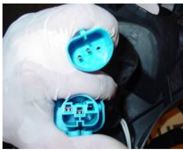
Step 10: Plug the supplied 2 to 1 wire harness into the new Anzo head light.
