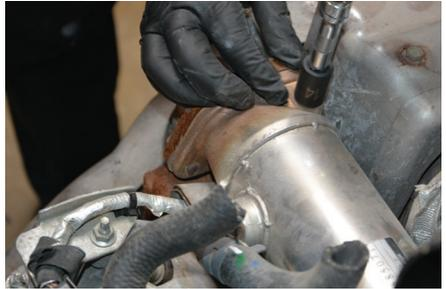
16. Move up EGR cooler out of the way by keeping it elevated.
