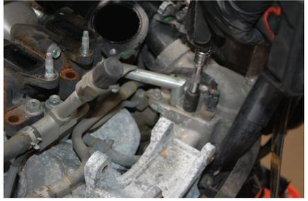
14. Disconnect EGR air intake (6 bolts and nuts). Move up and out of the way to make room for install.
