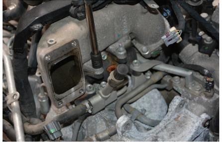
15. For LBZ models only: Remove top bolt from EGR cooler. For all other models remove all bolts.
