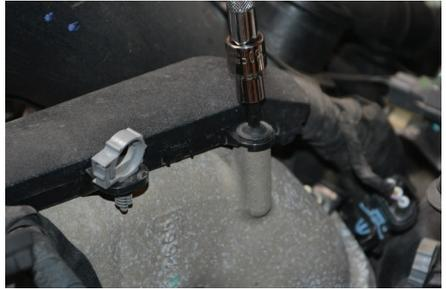
11. Remove Allen screws and nuts from air intake heater.
