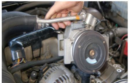
7. Remove opposite end of the high-pressure fuel line with a 17mm flare nut wrench. Set aside. The factory fitting will now be visible.
