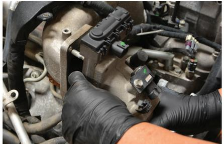
13. Remove high-pressure fuel line nuts and bolts from bracket on valve cover.
