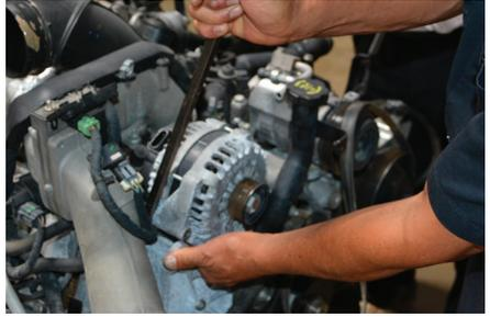
8. Bushing must be pulled forward, as shown, to allow space for longer PPE Ported Fuel Rail Fitting.
