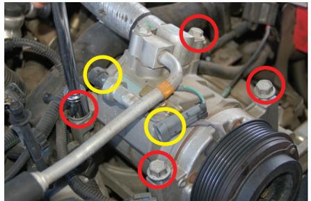
5. *Lift and move A/C compressor up and away.*
