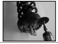
7. Locate the new front strut spacers. Install the new front strut spacers onto the strut and secure using the new 10 mm flange nuts. Make sure to use loctite and torque to 45 ft lbs.
