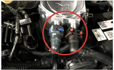
**NOTE:** *One of the post fittings is a larger diameter than the other. Be sure that you are connecting the fuel lines to the appropriate fittings (same as stock configuration). Excessive force should not be required for reconnecting the fuel lines.*
