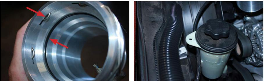
**NOTE:** Be careful not to damage the o-ring, intake air temperature sensor, or wiring harness during this step!
