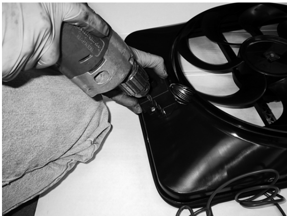
If necessary, drill two \frac{3}{16} " holes...
