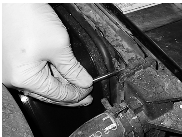
Install temp. probe near inlet hose...
