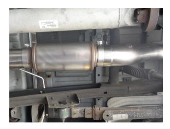
**Step 2.** Loosely install the muffler assembly as shown using the muffler clamp supplied and the muffler clamp previously used on the rear extension pipe. Adjust the pipes and muffler to fit properly and tighten the muffler clamps evenly using the torque specifications on page one of the instructions. Inspect the muffler clamps after 25-50 miles of operation and re-tighten if necessary.
