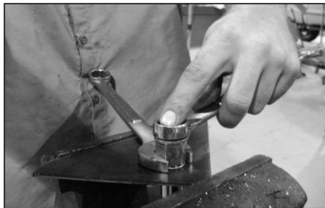
FIGURE 2 - 1/2" RIVET NUT SHOWN
