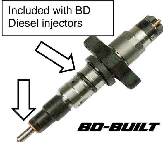
4. Install injector into cylinder head with male (high-pressure) connector port facing the intake manifold. Push down on fuel injector mounting flange to engage O-ring and seat injector.
