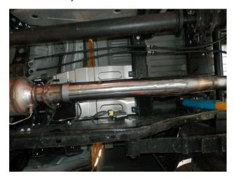
**Step 2.** Begin installation of the Magnaflow system by locating the indexing notch to the OEM peg then loosely clamping the Inlet Pipe Assembly to the outlet of the DPF using a supplied 4.00" clamp.
