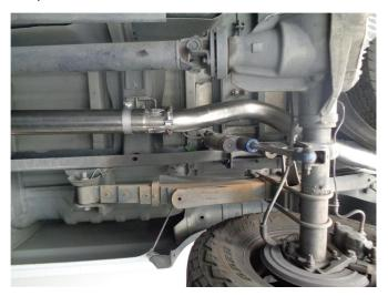
**Step 4.** Loosely install the Over Axle Pipe Assembly using the supplied clamp. Remove the sensor plug for 6.7L application. Loosely slip the Hanger Clamp Assembly over the pipe and locate the welded hangers to the rubber insulators.
