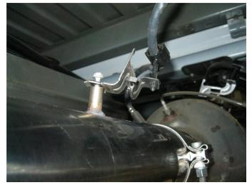
**Step 4.** For year spread 2013 and later with a long bed configuration attach the OEM cable bracket using the OEM bolt. This step is not required on other years or configurations.
