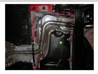
**Step 2.** Begin installation of the new system by attaching the Inlet Pipe to the factory outlet using the OEM clamp and fit the hangers into the rubber insulators. Leave all clamps loose until final adjustment.
