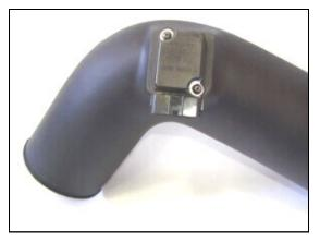
9. Using two  $8-32 \ge 1/2$ " button head screws (#10) install the factory M.A.F. sensor in the Airaid intake tube (#2) DO NOT USE THE **FACTORY SCREWS!**
