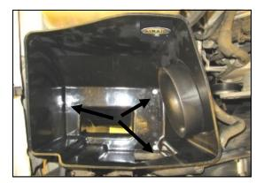
4. Using a 10mm socket, remove the five bolts and mounting plate from the engine compartment and set aside. Three of these bolts will be re used in step 6.
