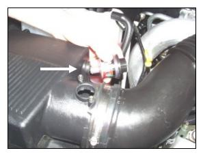
2. Remove the factory filter minder and grommet from the side of the factory airbox (save for reuse).
