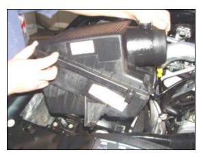
3. Remove the factory intake tube assembly from the engine. Rock the factory air box back and forth and remove it from it's mounting. There are only grommets holding it in, no bolts.
