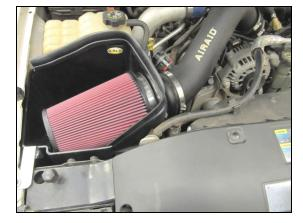
14. Install the Airaid Premium Filter (#1) onto the filter Adapter, and tighten the hose clamp. Install the Weather Strip (#7) onto the Airaid Cold Air Box. Reconnect the **M.A.F.** sensor wiring harness. (<u>Note</u>: Start from one corner and work your way around to insure proper alignment of the weather strip.)
