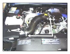
1. Disconnect the negative battery cable. A.) Disconnect the Mass Air Flow (M.A.F.) sensor wiring harness. Using the supplied T-20 Security bit, remove the two screws and the M.A.F. sensor from the tube (save the sensor for reuse). **B.**) Loosen the hose clamps on each end of the factory intake tube assembly.
