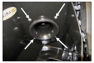
**8.**) Install four 1/4" button head bolts (#6), and four flat washers (#7) thru the **CAB** to secure the Airaid Intake Tube. Now tighten the three bolts at the bottom of the **CAB** and the two hose clamps on the hump hose.
