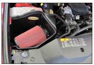
**11.** Install the Weather Strip (#5) onto the Airaid Cold Air Box. (*<u>Hint</u>: Start from one corner and work your way around for ease of install.*)
