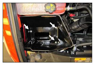
**4.** Install the Airaid Cool Air Box (CAB) (#3) into the vehicle as shown. Reuse three of the factory bolts
