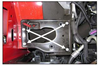
**3.** Using a 10mm socket, remove 4 bolts, and remove the factory air Box mounting plate.
