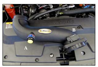
**6. A.)** Transfer the filter minder and grommet from the factory airbox into the Airaid Intake Tube
