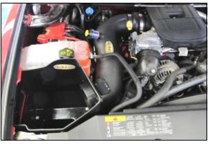
**7.**) Insert the Airaid Intake Tube into the **CAB** first, and then into the hump hose. Apply the Airaid Bubble Decal inside the Airbox as shown.
