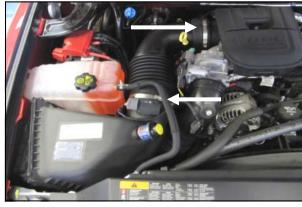
**1.** <u>Disconnect the negative battery cables.</u> Loosen the clamps on both ends of the factory intake tube and remove the tube from the vehicle.
