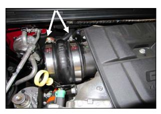
5. Install two #72 hose clamps (#9) onto the urethane
