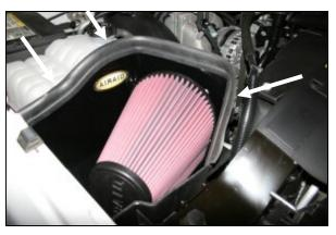
8. The Airaid Premium filter (#1) is a very tight fit in the CAB. For ease of installation, hold the filter in your right hand, and guide the bottom of the filter past the flange of the tube with your left hand inside of the CAB. It will fit! Tighten the hose clamp. Next install the weather strip (#5) on top of the CAB, starting at the fender and working your way towards the radiator.
