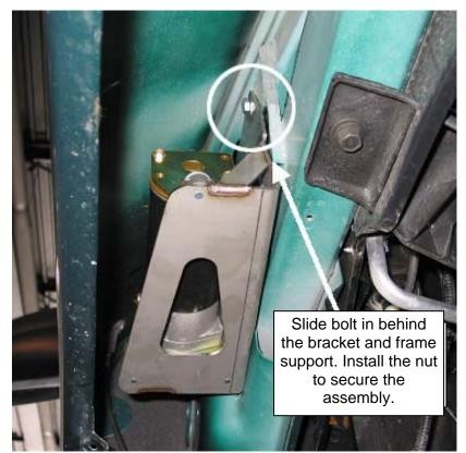
Tighten all bolts and secure assembly. Route the compressor pigtail wiring harness up towards regulator assembly the vou previously installed. You will also need to route a small section of plastic air hose from the quick connect fitting of the air compressor to the regulator assembly. Use the wiring diagram on page 11 as a reference for the wiring of the air hoses and the electrical wiring. NOTE: Be sure to keep all hoses and wiring harnesses away from any moving parts or heat sources.
