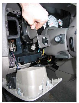
Install the switch into the newly drilled hole and secure it with a lock ring, then re-install the dash trim panels by reversing the removal procedure.
