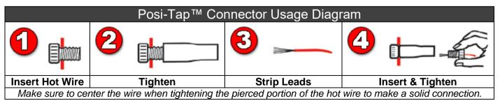
The ground terminals of the vehicle's batteries should be disconnected before performing any piercing/posi-tapping onto any ECM/PCM wire.
