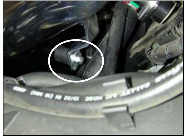
i. Align the intake pipe bracket with the rubber mount on the heat shield. Use the supplied washer and nylok nut and secure assembly.
