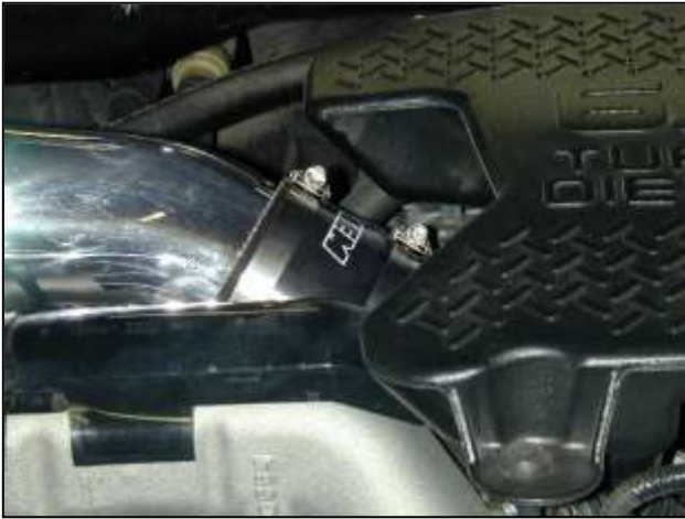
h. Install the intake pipe into the coupler on the turbo inlet hose.
