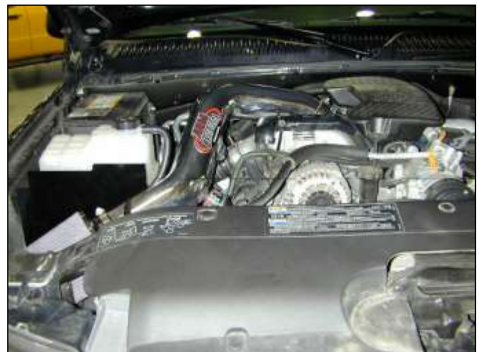
AEM® intake system installed
