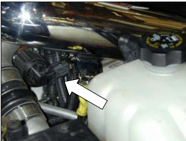
j. Reconnect the MAF sensor wire harness on the underside of the intake pipe.
