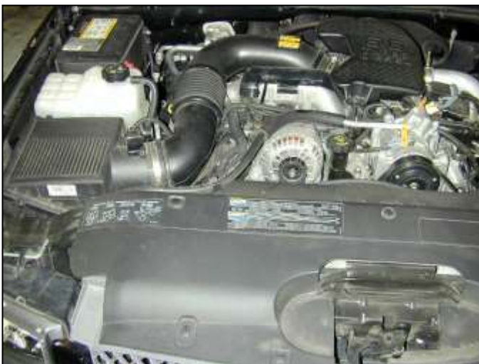
Factory air box system installed
