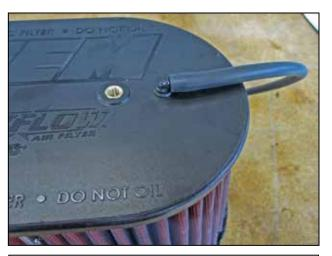
k. Install the small grommet (784631) into the drilled hole, and then install the 5/32" plastic elbow port (8-152) into the grommet. Install the 5/32" rubber air hose (5-3018) onto the elbow port as shown. This hose will be attached to the AEM® Filter Minder gauge at a later step.
