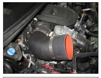
d. Loosely install another hose clamp (9472) over the outlet hose and install the intake elbow assembly onto the engine intake port as shown. Do not fully tighten the hose clamp yet.
