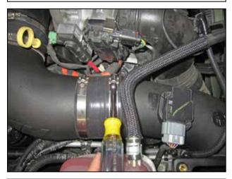
v. Tighten the hose clamp at the silicone hose connecting the lower intake tube to the intake elbow.
