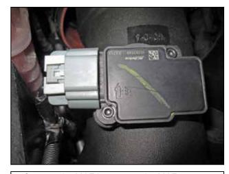
o. Connect the MAF harness to the MAF sensor and push the locking tab in to lock the connector.
