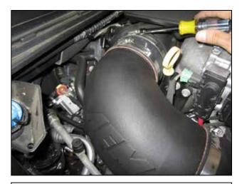
w. Fully seat the silicone hose at the engine intake port and tighten the hose clamp. The intake tube and filter installation is now complete. You are now ready to seal the air box.
