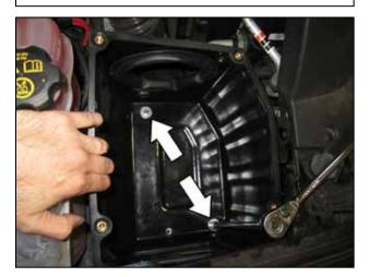
h. While pulling the air box toward the stock coolant reservoir to align the air box, install two of the M6 long bolts (1-2044) with two flat washers (08160) at the 2 mounting holes as shown. Make sure the air box inlet window is aligned with the stock air inlet window in the sheet metal fender liner. Tighten the two bolts.
