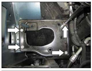
f. Using a 10mm socket, remove the 4 bolts retaining the stock air box mounting plate; remove the mounting plate.
