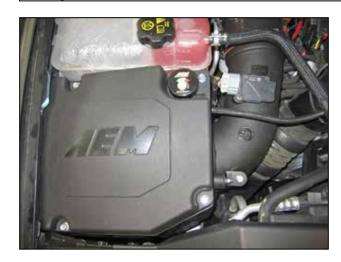
aa. Install the air box lid (9-0411) onto the air box (9-0406) as shown using the M6 hex/flange bolts (1-1016) provided. Start all 4 bolts by hand first and then tighten them with a 10mm socket to seal the air box.
