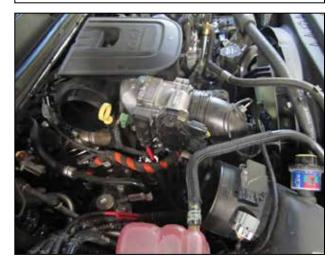
d. Remove the stock intake tube from the air box and engine air inlet.
