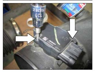
g. Using a T20 Torx bit, remove the 2 screws retaining the MAF sensor to the upper air box lid. Remove the sensor for use with your new AEM® cold air intake. Make sure the O-ring is intact on the sensor.
