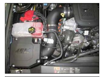
AEM® intake system installed.
