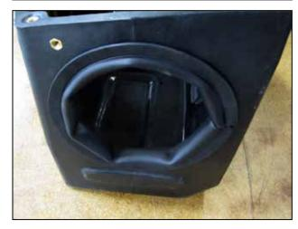
e. Install the bulb seal (102494) around the inside edge of the outlet hole of the air box (9-0406) as shown. Trim any excess bulb seal as needed.
