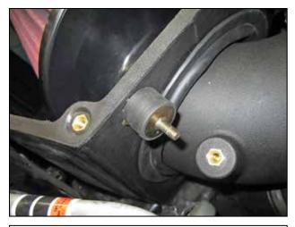
r. Install the rubber mount (1228598) into the M6 brass insert on the side of the air box as shown. Tighten by hand.
