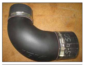
c. Install the silicone hose (5-1066) onto the outlet end of the intake elbow (9-0412), on the "A" side of the AEM® logo. Install the larger silicone hose (5-450) onto the inlet side of the intake elbow, the end closest to the "M" in the AEM® logo. Secure both couplers with (9472) hose clamps as shown.
