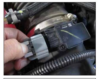
b. Depress the snap tab on the connector as shown and pull it to disconnect the harness from the MAF sensor.
