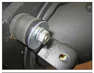
s. Loosely install the "L" bracket (32-3087), one flat washer (08160), and one M6 serrated nut (444.460.04) onto the rubber mount.
