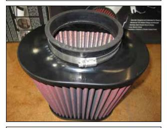
I. Install the filter insert (5-2279) into the outlet of the Dryflow™ air filter. Install the large hose clamp provided over the air filter outlet as shown.
