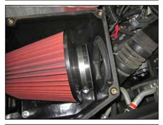
m. Insert the Dryflow™ air filter assembly into the air box as shown.
