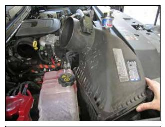
e. Pull up on the stock filter air box starting on the side closer to the engine to "pop" it free from its mounting grommets. Remove the air box assembly from the engine bay.
