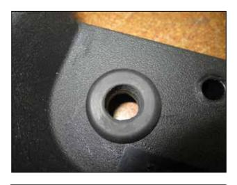
x. Install the grommet (784642) into the 0.75" hole in the corner of the air box lid (9-0411) as shown.
