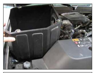
g. Place the air box into the engine bay where the stock air box was located as shown. Make sure the new left front mounting grommet is aligned with the threaded hole in the engine bay.
