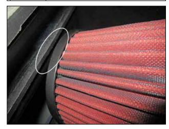
u. Rotate the lower intake tube and filter assembly until the edge of the filter cap lines up with the top edge of the air box opening near the fender as shown.
