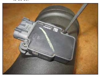
b. Install the MAF sensor onto the MAF pad on the lower intake tube (9-0405). Secure with the two 4mm Allen bolts provided. Tighten the bolts.
