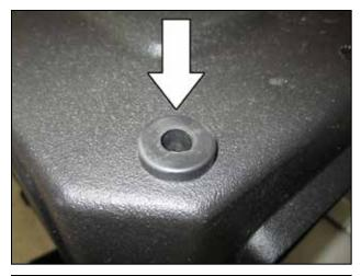
f. Install the foot grommet (784647) on the outside of the air box in the larger left front mounting hole as shown.
