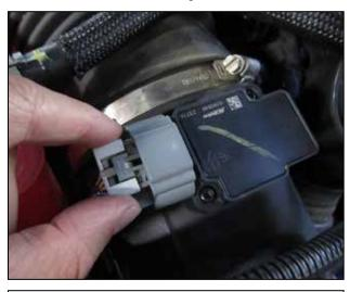
a. Pull back the grey locking tab on the female MAF sensor connector to unlock it.
