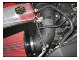
n. Loosely install the (9-0405) lower intake tube through the bulb sealed outlet hole in the air box and into the Dryflow air filter base adapter as shown.
