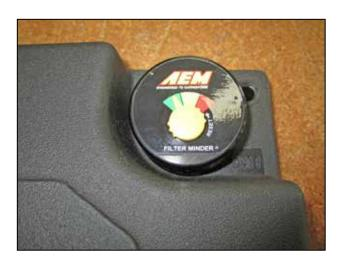
y. Install the filter minder gauge (35-80321) into the large grommet. Use glass cleaner to lubricate the hole in the grommet if needed.
