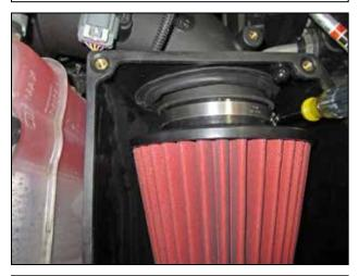
p. Fully seat the Dryflow air filter onto the lower intake tube inlet and align it inside the air box as shown. Tighten the large hose clamp at the filter base.
