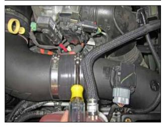
q. Install the fourth hose clamp (9472) on the open silicone hose already mounted on the intake elbow. Insert the outlet end of the lower intake tube (9-0405) into the silicone hose. Loosely secure the hose clamp so the intake tube can rotate inside the hose.
