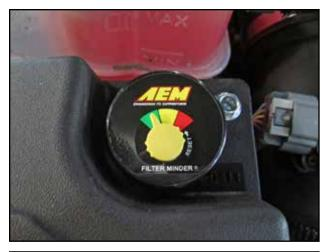
ab. Make sure the AEM® filter minder gauge needle is pointing to the green sector. Once your Dryflow filter is dirty and the pressure drop (restriction) across it reaches 20 inches (of H2O), the gauge needle will point to the red sector. This will mean it is time to wash your reusable AEM® Dryflow™ air filter.
