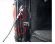
Step 1: Locate the two t27 screws and remove them.
