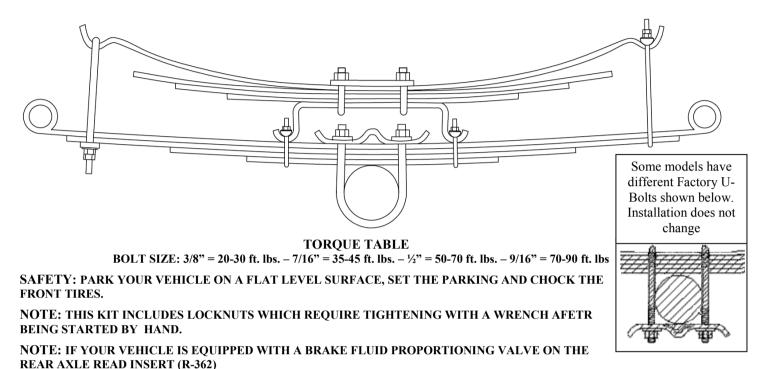
NOTE: Your spring may have a small hole in the end, this is for our manufacturing process and will not be used. IMPORTANT NOTE: IF YOUR VEHICLE IS EQUIPED WITH A FACTORY CONTACT OVER LOAD IT MUST BE REMOVED BEFORE INSTALLING THE NEW HELPER SPRINGS.
