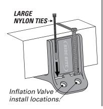
Select a protected location to install the Inflation Valves, such as the bumper or the body of the vehicle.
