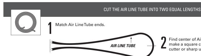
Find center of Air Line Tube, make a square cut with tube cutter or sharp utility knife.
