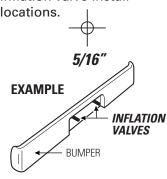
Install Inflation Valve assembly as shown.
