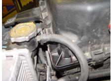
**Note:** Top bracket on passenger's side secures wiring loom. Find alternate mounting point near by and resecure. The 2 top brackets & 1 bottom bracket.
