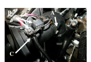
A) Slide the rubber elbow over the Airaid filter adapter, install one #80 hose clamp (#20), and tighten the hose clamp. **B**) Using three 8-32x1/2" button head screws (#13), reinstall the factory Mass Air Flow sensor, and temperature sensor into the Airaid filter adapter. Do Not Use The Factory Screws! C) Reinstall the wiring harness anchor into the hole in the filter adapter just below the temperature sensor.
