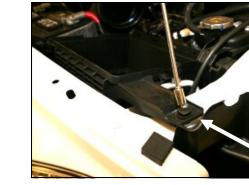
**3.** Using a 10mm socket, remove the nut that holds the front of the airbox base and grommet assembly to the radiator support.
