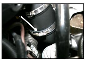
14. Tighten the factory hose clamp where the Airaid metal tube slips into the factory rubber elbow on the turbocharger.
