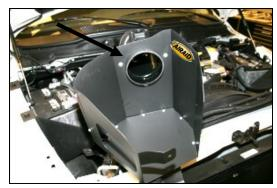
**10.** Assemble the Cool Air **D**am panels as shown using the seven 6-32x5/16" screws (#8), #6 flat washers (#9), and keps nuts (#10). Next install the Airaid filter adapter thru the CAD panel using three 1/4-20x1/2" button head bolts (#11), and 1/4" flat washers (#12). (See Arrow) Apply the Airaid Foil Decal onto the Panel as shown.
