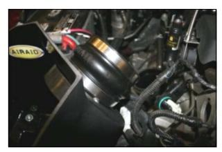
**10.** Install the supplied hump hose (#5) onto the filter adapter using two #72 hose clamps (#17). Leave the clamps loose for now.
