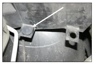
7. Install the supplied well nut into the factory airbox mounting hole closest to the fender as shown.
