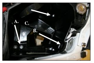
9. Install the CAB into the vehicle as shown. A.) Install the 3/8" button head bolt and flat washer thru the **CAB** and into the well nut. **B**.) Install the 6mm x 25mm hex bolt and flat washer thru the CAB and into the captured nut in the fender. C.) Install the 5/16" bolt flat washer, and flange nut thru the CAB and L-bracket. Tighten all mounting bolts at this time.
