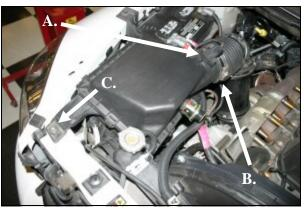
1. Disconnect the negative battery cables. A.) Using the provided T-20 torx bit, remove the two temperature sensor mounting bolts and the sensor from the factory intake tube (set aside for reuse). **B**.) Loosen the hose clamp where the flexible tube connects to the factory airbox lid. C.) Using a 10mm socket, remove the nut that secures the factory airbox to the radiator mount.
