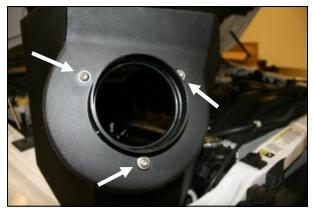
8. Install the filter adapter into the Cool Air Box using three 1/4" Button Head bolts and flat washers as shown.
