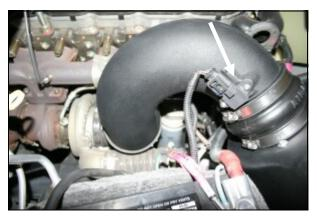
**11.** Install the Airaid Intake Tube (#2) into the factory turbo elbow and then into the hump hose. Adjust for fit, and then tighten all three hose clamps. Reinstall the intake temperature sensor into the Airaid Intake Tube using two 8-32 button head screws (#7) and #8 flat washers (#8). **Do Not Use The Factory Screws!**
