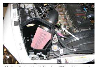
**12.** Install the Airaid Premium Filter (#1) onto the filter adapter and tighten the clamp. Install the weatherstrip onto the top of the **CAB** starting at the right fender and working your way towards the radiator. Next reinstall the factory filter minder and grommet into the Airaid Intake Tube. Apply the Airaid Decal as shown.
