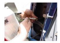
Step 8: Connect the resistor to the taillight housing.
