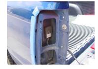
Step 6: Place the resistor in a safe location in the housing.
