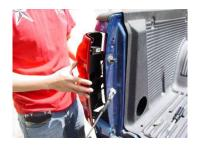
Step 3: Remove the taillight by pulling straight out.
