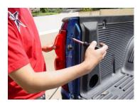
Step 1: Lower the tail gate exposing the two screws.
