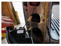
Step 7: Plug the resistors in and the wire harness into the circuit board under the bed.
