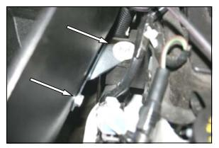
**8.** Reinstall the factory bolt that was removed in step #3, through the bracket that is bolted onto the side of the Cool Air Box. Adjust the box for fit, and tighten both bolts.
