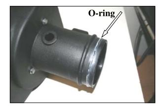
**4.** Install the adapter gasket (#12), and filter adapter (#4) into the Airaid Cool Air Box (#2) using three 1/4-20x5/8" hex bolts (#6), and 1/4" flat washers (#7).
