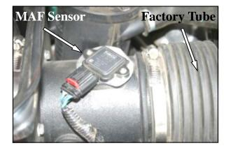
10. Install the MAF sensor into the Calibration Plate on the Cool Air Box using two 8-3/8" button head bolts (#9), as shown. Reconnect the MAF sensor wiring harness.
