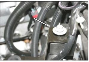
**3.** Remove one bolt from the factory airbox mounting plate, and save it for reinstallation in step #8.
