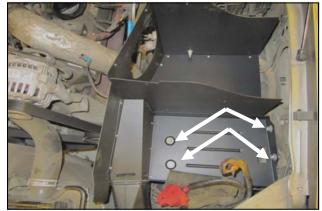
8. Place the CAD assembly in the engine compartment and start the four factory bolts from step 4. Leave the bolts loose for now.
