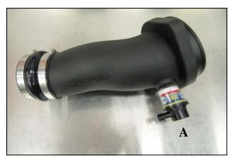
9. Create the Tube assembly. A.) Transfer the factory grommet and filter minder into the Airaid Intake Tube (#2). **B**.) Slide the Hump Hose (#10) and Clamps (#13) onto the Tube as shown. Leave the clamps loose for now.
