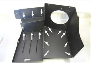
5. Create the Cool Air Dam, or CAD assembly as shown using the Bottom Panel (#3), Side Panel (#4), and
