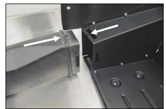
7. Transfer the air inlet from the factory airbox assembly into the CAD assembly. The air inlet has an indexing tab that mates with a slot in the Panel. NOTE: Vehicles built ``BEFORE 12/7/98" do not have this air inlet design. This intake can be used with or without the factory inlet. It is available from Ford as a special order part. Ford Part number:
