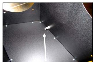
6. Transfer the air temp sensor from the factory airbox into the CAD assembly
