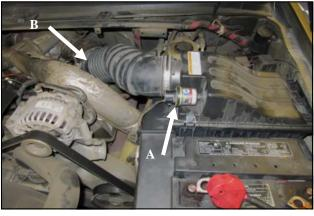
2. A.) Disconnect the filter minder in the top of the airbox.
