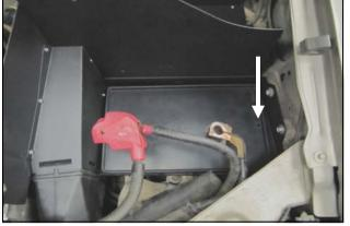
**14.** Place the Battery Mat (#7) into the **CAD** assembly with drain tube on the Drivers side.
