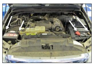
1. Disconnect the battery cables. Disconnect both the Drivers side and Passenger side battery cables.
