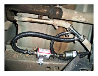
(Fig. 15) Vent Fill Neck Adapter installed.
