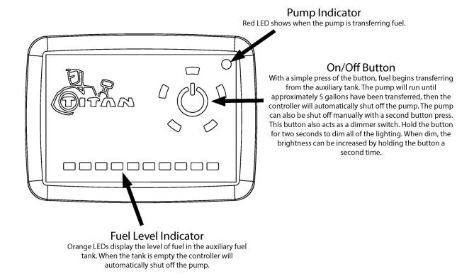
(Fig. 25) Operation instructions for TITAN™ Electronic Fuel Controller.
