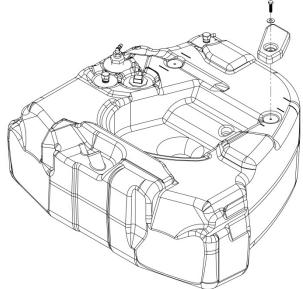
(Fig. 8) Connecting small eyelet end of grounding wire to top of electric fuel sensor. Other end attaches to chassis frame
