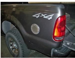
(Fig. 16) Fuel Door located in outside fender.
