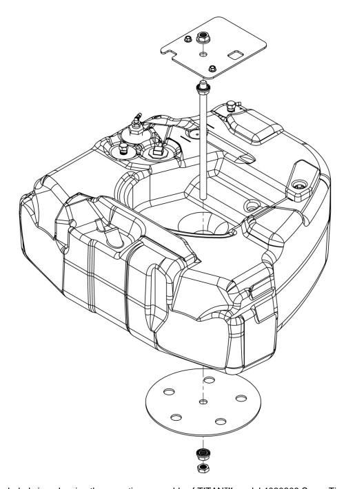
(Fig. 1) Exploded view showing the mounting assembly of TITAN™ model 4020208 Spare Tire Auxiliary Fuel System (STAFS) 30 gallon tank.
