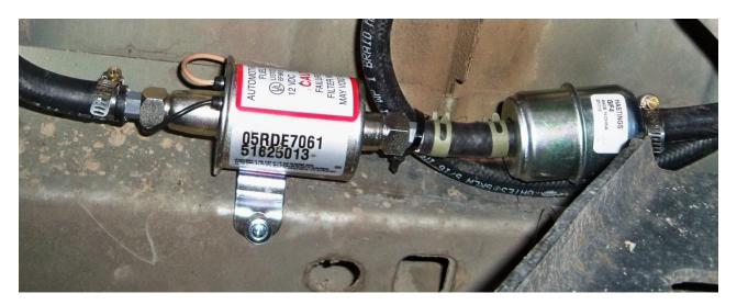
(Fig. 14) Fuel pump and inline filter installed.
