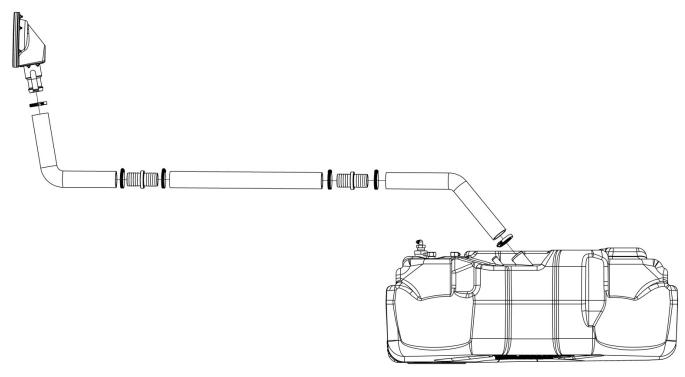
(Fig. 11) Exploded view of the rear of the STAFS tank (side of tank nearest the rear bumper) showing the fill hose plumbing schematic. A 5/8" vent hose running from the vent barb on the tank to the barb on the Poly Filler Neck Flange Assembly is not shown in this view.
