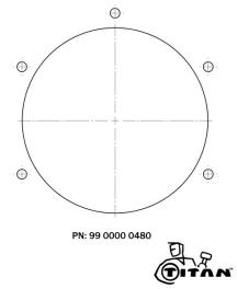
(Fig. 21) Facsimile of template supplied for Fuel Door installation in outside of fender.
