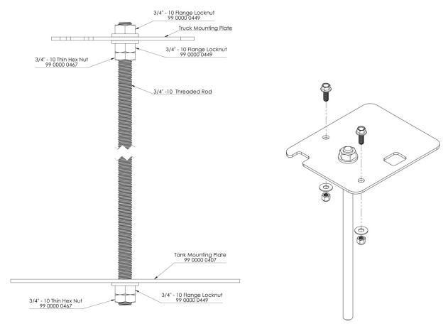
(Fig. 4) Side view of tank mounting plate assembly, threaded rod, and bottom tank mounting plate. Be sure to torque the nuts on the top plate to 45 ft. lbs, the flanged nut on underside of Tank Mounting Plate to 15 ft. lbs. against the tank and the jam nuts ("Thin Hex Nut") at the plate and very bottom to 45 ft. lbs.
