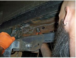
(Fig. 13) Using a hammer to bend sheet metal edge out of the way.
