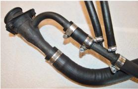
(Fig. 7) Vent, Fill Neck Adapter installed in the vent line of the fill neck of the stock, OEM, midships tank. Install so the larger,3/8" barb is farthest away from the fill neck. Adapter is to be installed so the two hose barbs point toward the filler neck cap as shown.
