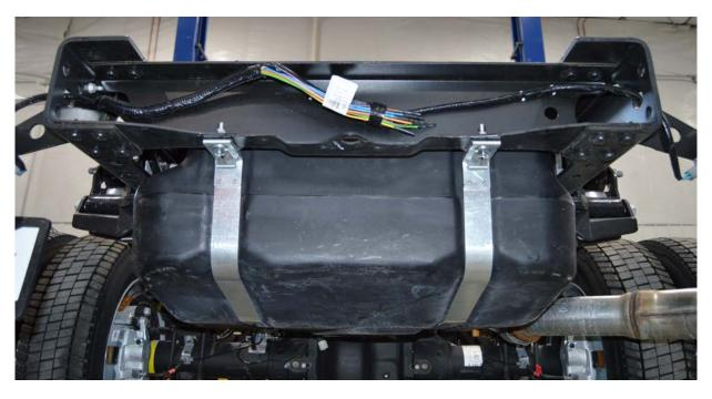
(Fig. 3) Rear of vehicle, showing how tank straps are attached to the frame.
