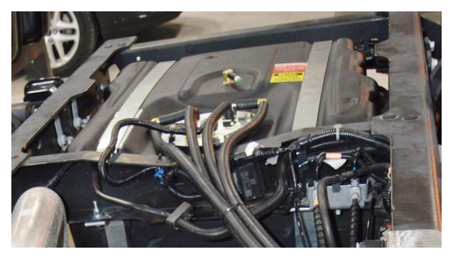
(Fig. 4) Front of TITAN tank, showing how tank straps are attached to the frame. The tank product shown is the same tank in a different application, but the attachment to the frame is correct for this auxiliary product too.
