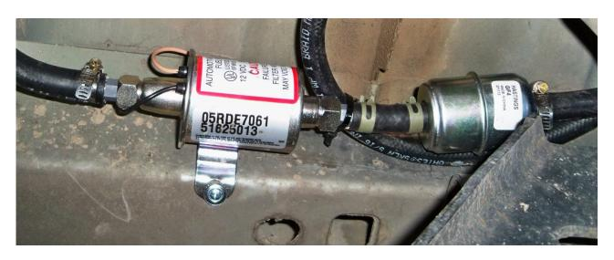
(Fig. 8) Fuel pump and inline filter installed.
