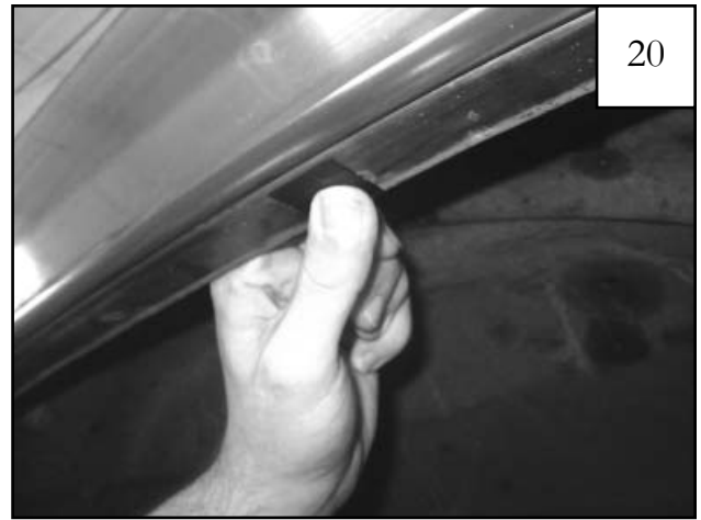
Remove flare. Center a supplied Tab (MT1-0002) over the marks made in step 17, aligning edge of tab with inside edge of fender lip (tab may extend over outside of fender).
