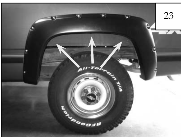
Ensuring flare is properly located on fender, start supplied screws (SW1-0050) through each of the remaining holes.
