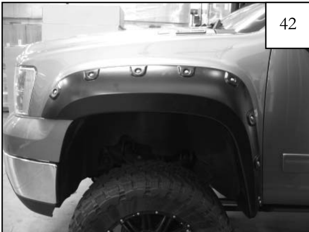
Reinstall wheel. Completed front flare installation.
