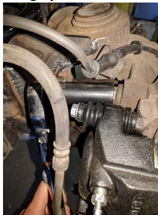
Figure 2. Removing Brake Caliper Carrier Bolts
