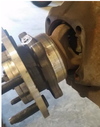
Figure 6. Removing Unit Bearing/Hub and Axle Assembly from Axle
