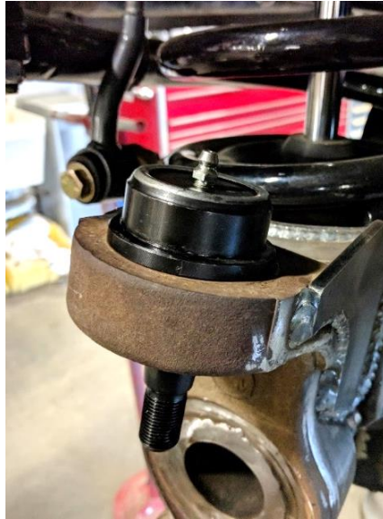
Figure 12. Upper Ball Joint Pressed In
