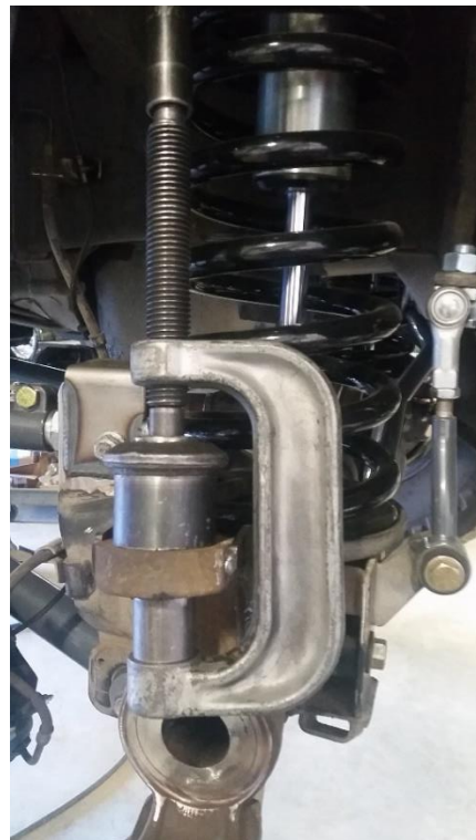
Figure 9. Pressing Out Upper Ball Joint
