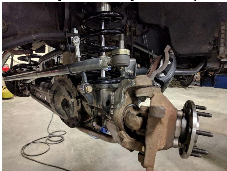
Figure 4. Tie Rod Removed
