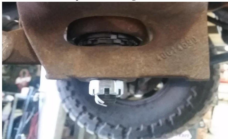
Figure 14. Cotter Pin Installed
