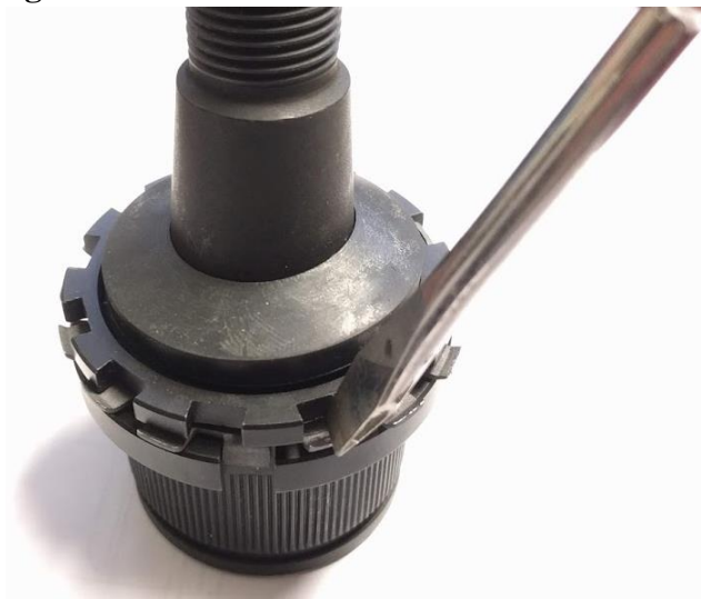
Figure 18. Bending Locking Tabs Back
