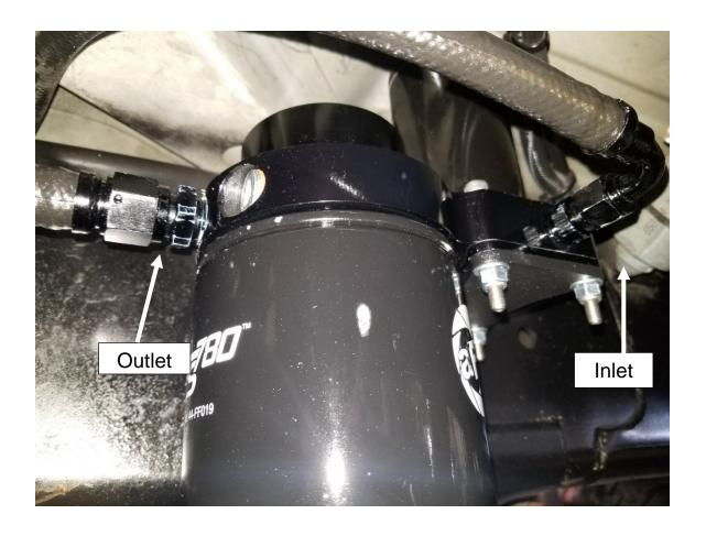
15. Attach the fittings to the inlet & outlet ports of the fuel manifold assembly. Make sure all connections are tight.
