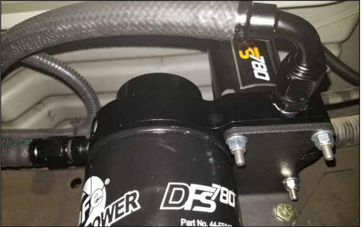
Step 13: Attach the fittings to the inlet & outlet ports of the DFS 780 Pro fuel pump. Make sure all connections are tight.
