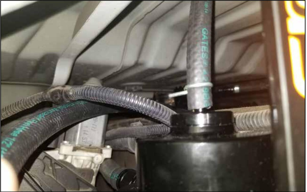
Step 15: Carefully route the 1/4" hose to the DFS780 Pro fuel pump, making sure not to kink the hose or allow it near moving parts. Carefully mark and then cut the hose to the correct length. Using the supplied 7/16" spring clamp, attach the hose to the nipple on the top of the air chamber on the DFS 780 Pro fuel pump assembly.
