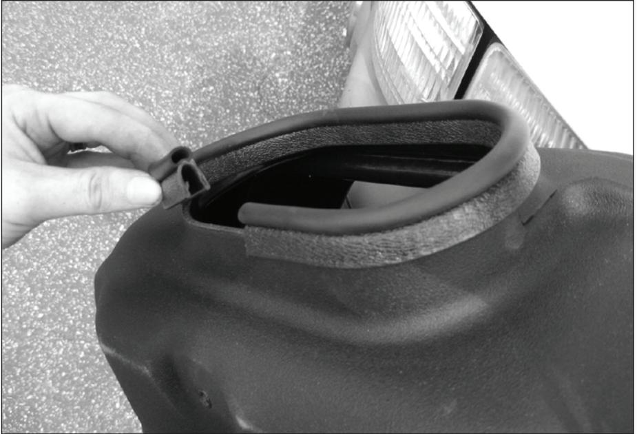
**8.** Install Banks filter hose clamp (Item 8) onto the Banks filter cuff (Item 2). Place Banks Filter into Banks filter housing.
